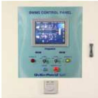
The monitor & control panel is PLC based and configured to activate and deactivate UV lamps via UV power supply panels in order to maintain the sufficient UV dose while conserving power.
